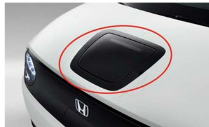
Charge port in the hood
