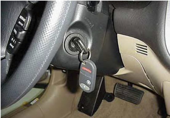
Turning the ignition key to the OFF position stops the flow of electricity in the cables.
