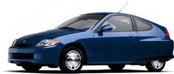
2000-2006 Insight models are 2-passenger cars with a distinctive aerodynamic shape and rear fender skirts.
