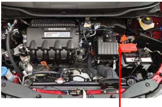
Positive Battery Terminal
