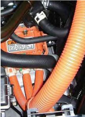
High-Voltage Cable Connection to Motor
