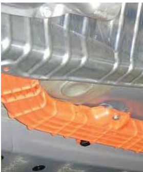
Electrical shield bolted to undercarriage
