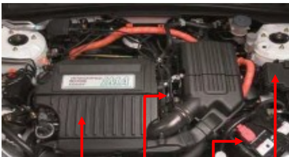
Engine Motor 12-Volt Battery Under-hood Fuse Box
