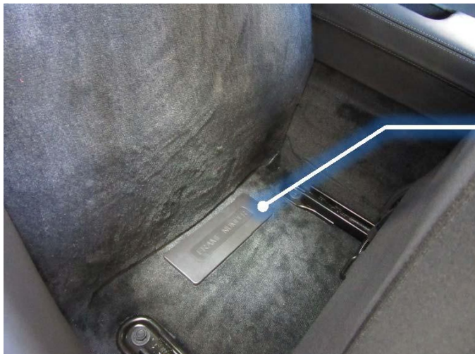
Stamped into the floor panel behind the passenger seat under a plastic panel marked FRAME NUMBER
